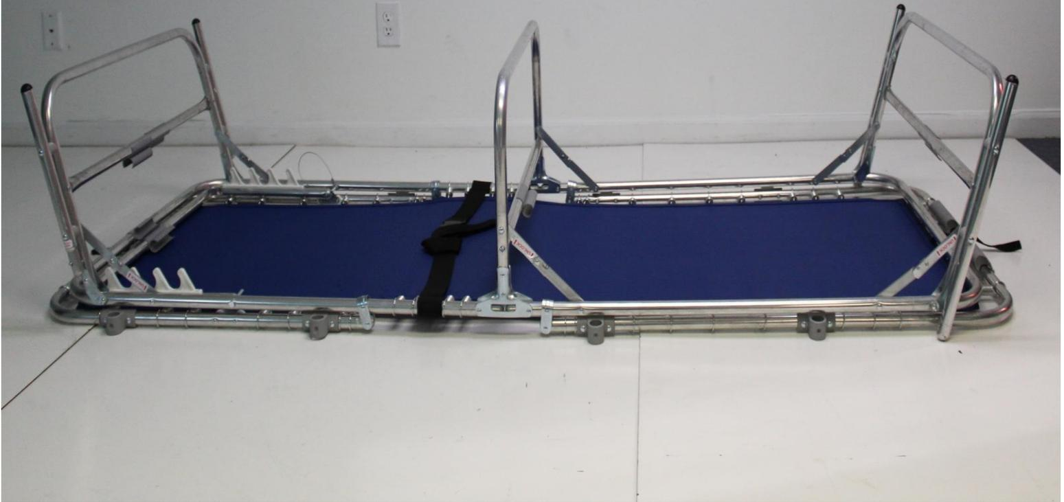
5. Rotate Westcot to the standing position, dress the Mattress across the Decking Platform, and secure Mattress to frame with the Velcro Straps.
